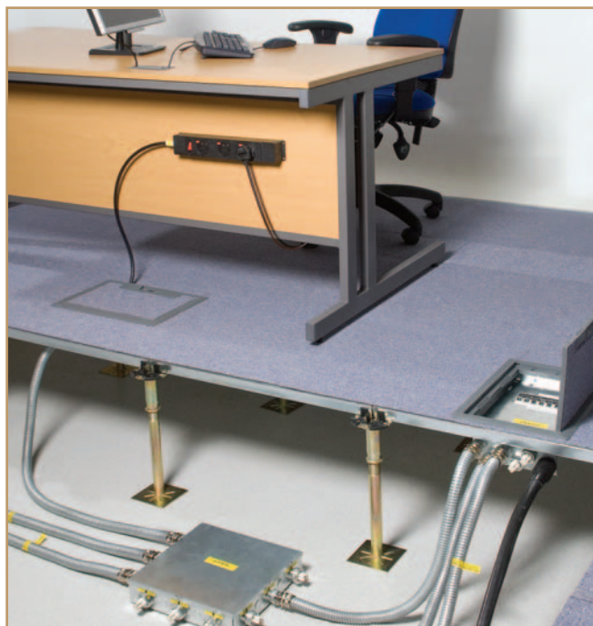
The complete solution from SWA infeed. MT32 Underfloor pre-wired plug and play system feeds desk modules via an MT32 Master Distribution Unit and Floor Box
