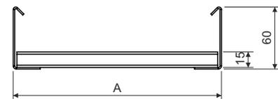
configuration: PO - Pre-Galvanized, zinc-layer 15 - 27 µm
