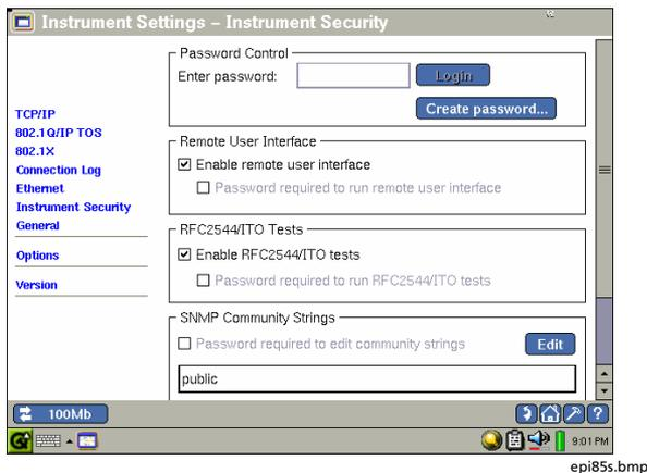
**Figure 22. Instrument Settings–Security Screen**
