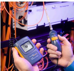
Figure 1. Dirty fiber end-face as seen through a FiberInspector video microscope.
